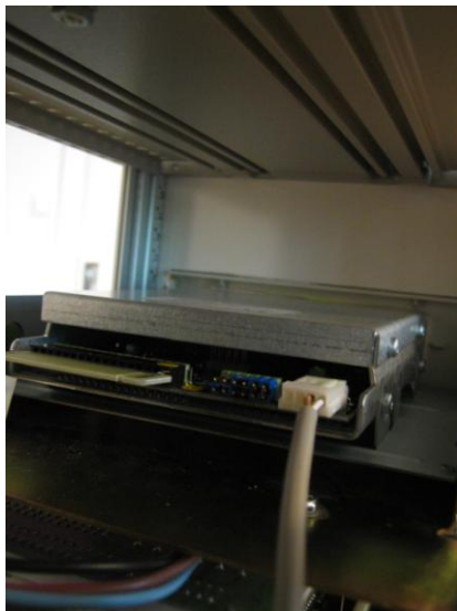
Figure 20 Connect the power cable to the DDR unit.
