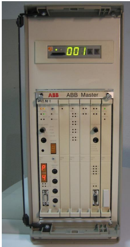
Figure 1 DDR unit of type NDDD 002 mounted in a MasterView 830 cabinet.
