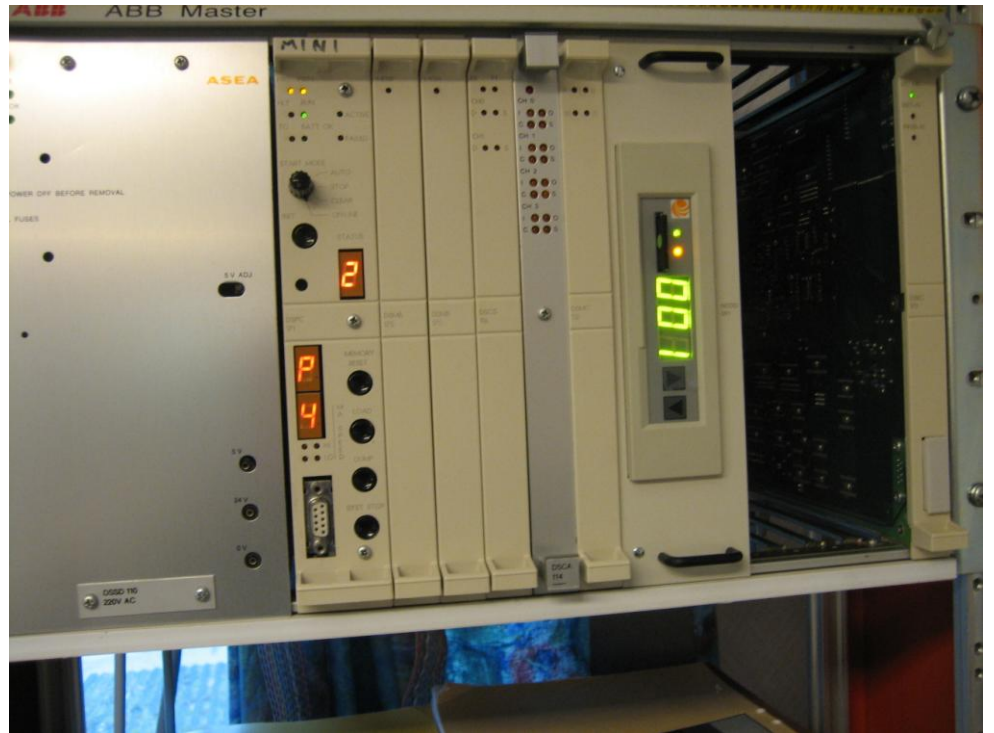
Figure 16 The NDDD 001 unit is busy, Busy LED in On.
