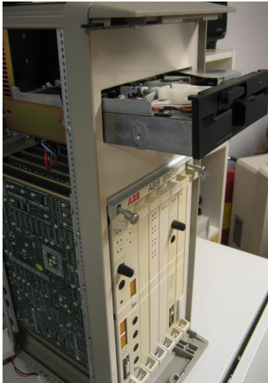
Figure 19 Remove the old DSMD floppy unit for the MasterView cabinet.
